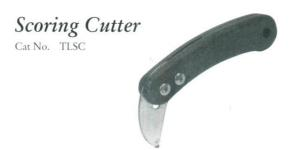
Handle is contoured for correct grip. Reversible double ended blade is carbide tipped to allow an easy break along score line. Ideal for use on all plastic laminates as well as wonder board.
